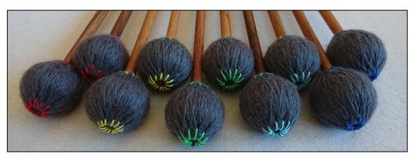
Heavy poly ball cores Ø 30mm with rubber coatings of varying hardness. Hand wrapped with a yarn blend of 75% wool 25% acrylic for warm sound and good durability. Tight wrap for clear and direct attack. The softer models have a multitone effect which makes them sound softer at lower dynamics and harder at higher dynamics. Waxed beech wood handles, Ø 8mm, length 42cm.
