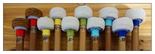
The heads of these mallets consist of stacked layers of fabric or leather, held together by a threaded nylon rod that is securely glued to the bamboo shaft. The nylon thread is much more durable and resilient than wooden threads. The upper nut can be tightened or loosened on all models to vary the number of layers or the hardness of the head.
